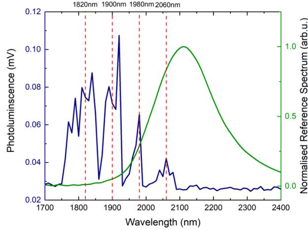
Figure 4 Resonance spectrum of the NW-microstadium cavity in blue. The free spectral range of the peaks is 80nm, with a very strong resonance depth. In green is the PL of an ensemble of NWs of the same sample to show the overlap between the spontaneous emission and the stimulated emission spectrum
