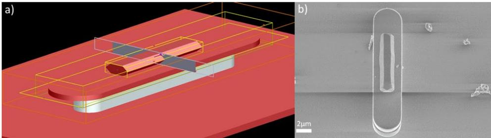
Figure 1 a) Schematic of the NW-microstadium cavity which was used to achieve stimulated emission. b) SEM image of a fabricated NW-microstadium cavity.
